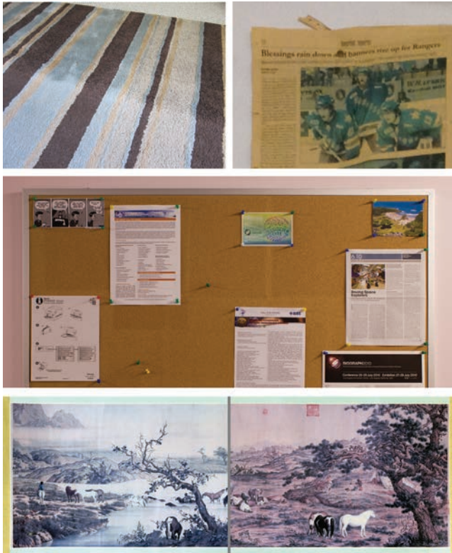
Fig. 2. Photographs depicting scenes in which fading due to light exposure has taken place. Top Left: An area rug has faded everywhere except where a couch had been placed. Top Right: A newspaper has turned yellow from many years of light exposure. Middle: Printed materials have been added and removed from a bulletin board over time, resulting in an irregular fading pattern. Bottom: The left end of a mural has been exposed to more light than the right, yielding uneven fading along its length. Photographs of the two ends are shown adjacent to one another so that the difference is clearly visible.
